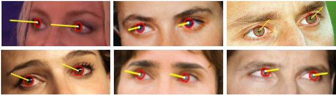
Figure 12: Reconstructed 3D eye gaze results with varying view directions and eye colors. Our system detects the iris and pupil region (red) and estimates the 3D eye gaze (yellow).
